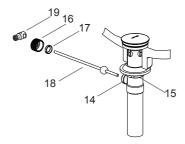
Remove the latch(19) and retaining nut(16). Fit the plastic washer(17) and retaining nut onto the ball lever(18). Insert the ball lever assembly into the drain lever hole and through the stopper hole. Tighten the retaining nut.
